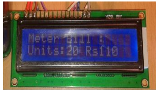
Fig 5.LCD display of Energy meter consumed units with bill
