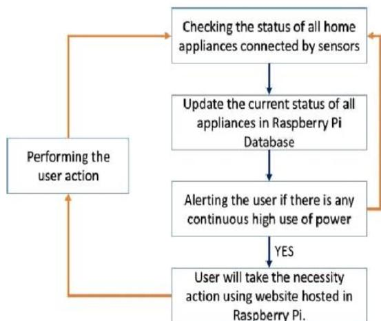
Fig 4. Algorithm showing raspberry pi working system
