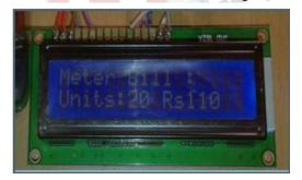
Fig 6.LCD display of Energy meter Consumed units with bill
