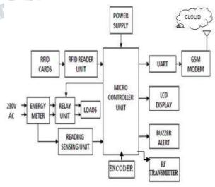
Fig: 1Proposed block diagram of Transmitter
