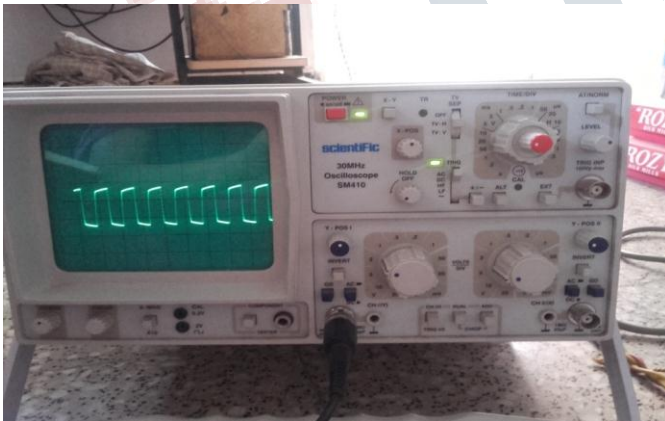
Fig 9: Schmitt Trigger output
