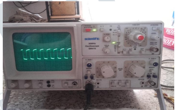
Fig 7: Schmitt Trigger output.
