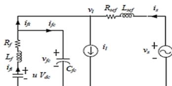
**Fig. 5: Single phase equivalent circuit of DSTATCOM topology with foreign inductor in distribution system.**
