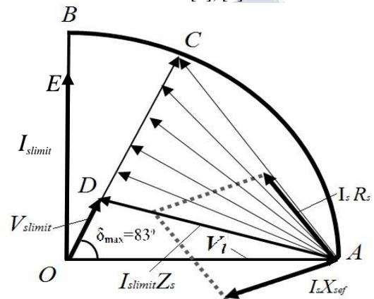
**Fig. 6: Voltage regulation performance of DSTATCOM with foreign inductance.**
