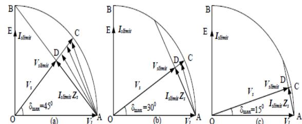
**Fig. 4: Voltage regulation performance curve of DSTATCOM at different  $R_s/X_s$ s. (a) For  $R_s/X_s = 1$ . (b) For  $R_s/X_s = \sqrt{3}$ . (c) For  $R_s/X_s = 3.73$**
