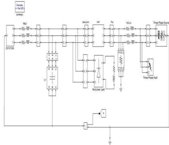
**Fig. 8: Simulink Models of distribution system with DSTATCOM and proposed foreign inductor**
