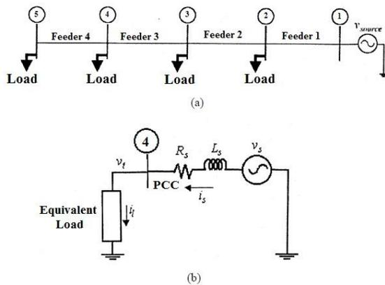
**Fig. 1: (a) Radial system under test and (b) its Thevenin equivalent at bus 4.**
