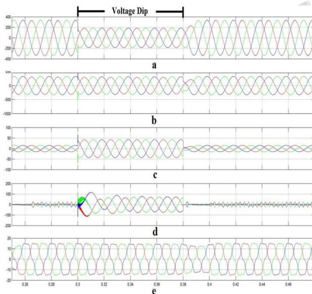
**Fig. 11: Voltage regulation performances of DSTATCOM during voltage dip with proposed plan. (a) PCC voltages. "V" (b) Load Voltages. "V" (c) Source currents. "A" (d) Filter currents. "A" (e) Load currents. "A"**
