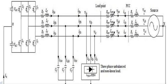
**Fig. 2: Three phase equivalent circuit of DSTATCOM topology in distribution system.**
