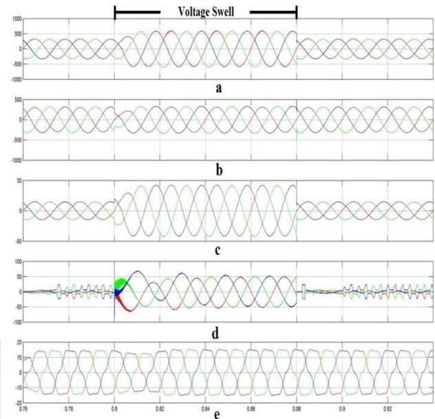
**Fig. 12: Voltage regulation performances of DSTATCOM during voltage swell with proposed plan. (a) PCC voltages. "V" (b) Load Voltages. "V" (c) Source currents. "A" (d) Filter currents. "A" (e) Load currents. "A"**
