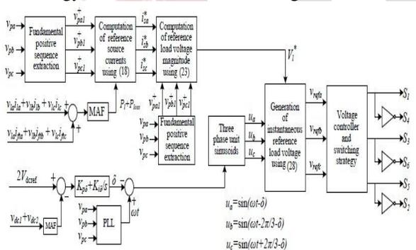
**Fig. 7: Block diagram of proposed multifunctional control strategy**
