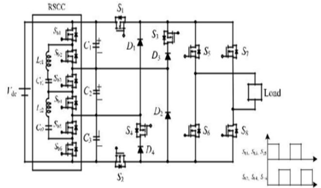
**Fig. 12. Proposed multilevel inverter with RSCC**
