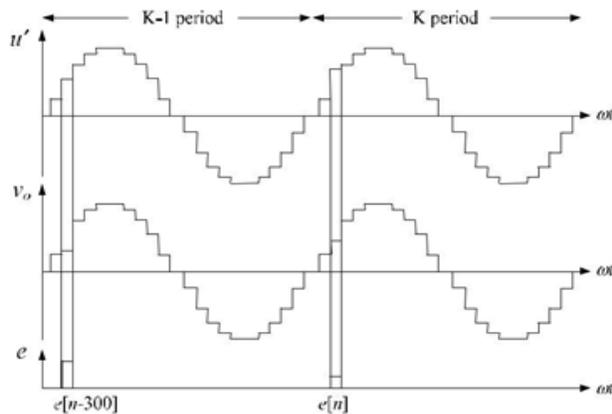
**Fig. 16. Schematic of modified SPWM**
