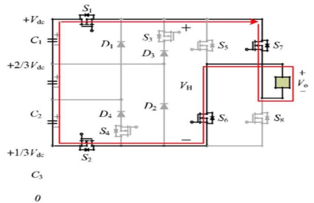
Fig. 8. Switching combination of output voltage level  $-V_{dc}$
