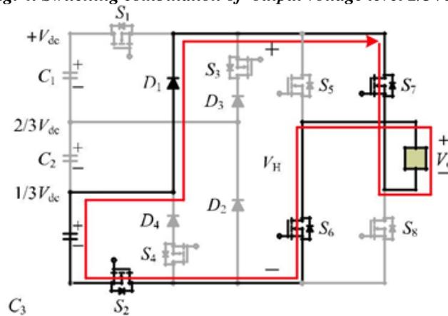
Fig. 6. Switching combination of output voltage level  $-1/3V_{dc}$
