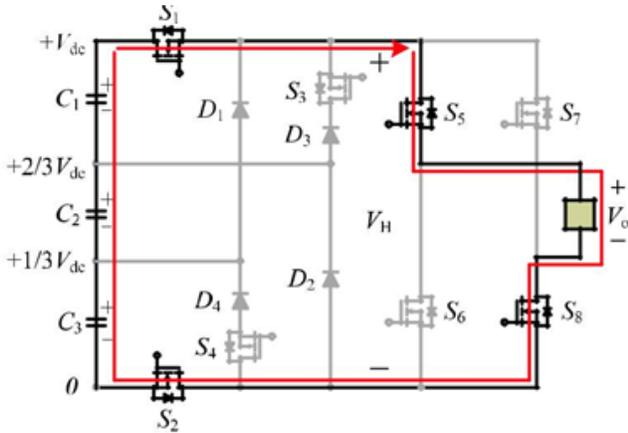
Fig. 4. Switching combination of output voltage level  $2/3V_{dc}$
