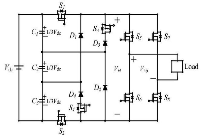
Fig. 2. Proposed seven-level inverter topology
