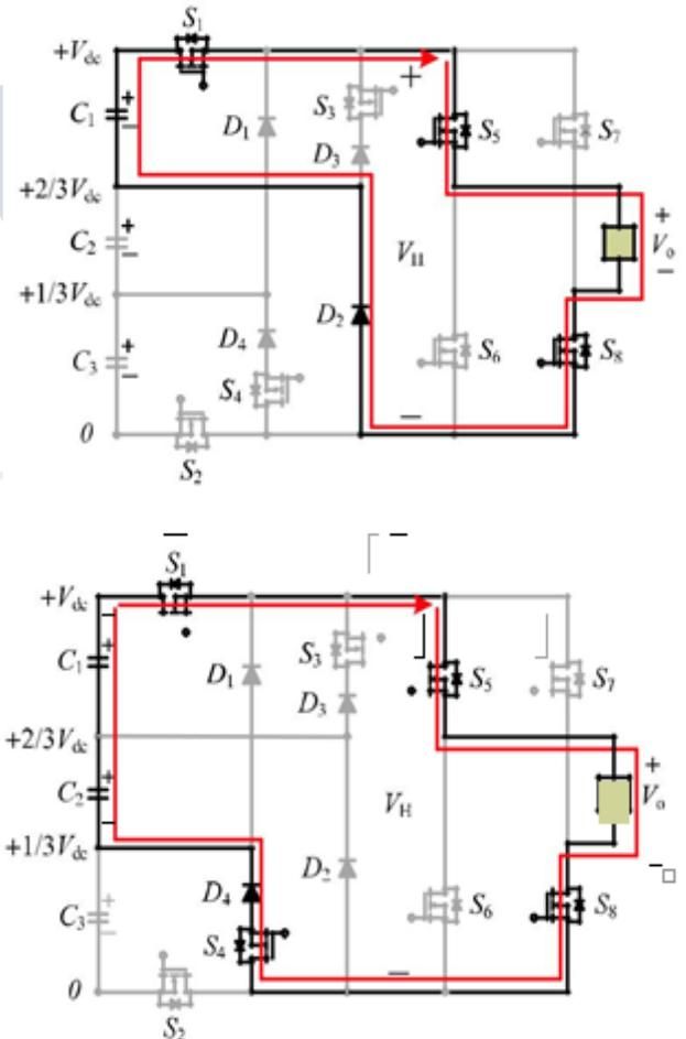
Fig. 3. Switching combination of output voltage level  $1/3V_{dc}$ .
