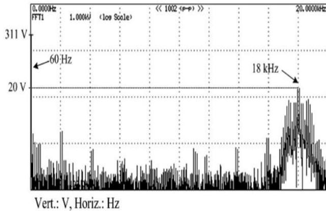
**Fig. 19. Output voltage harmonic spectrum of  $v_{ab}$  calculated by FFT**
