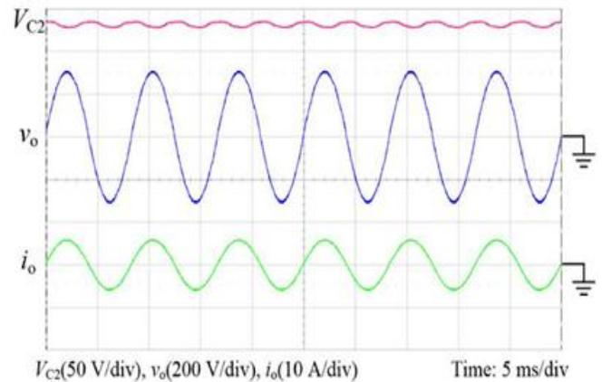
**Fig. 21. Waveforms of  $v_{C2}$ ,  $v_o$ , and  $i_o$  at 1000 W**
