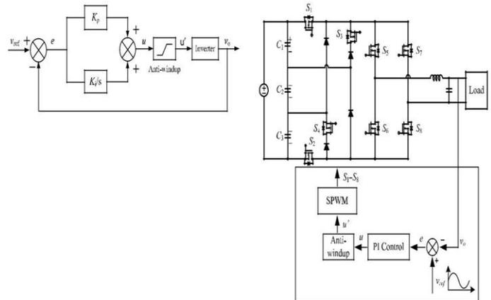
**Fig. 14. Block diagram of PI control**
