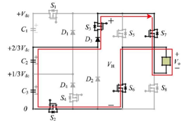
Fig. 7. Switching combination of output voltage level  $-2/3V_{dc}$
