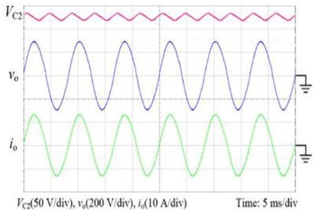
**Fig. 22. Waveforms of  $v_{C2}$ ,  $v_o$ , and  $i_o$  at 2000 W.**
