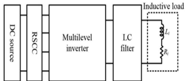
Fig. 23. Test block diagram of inductive load Fig. 24 shows the output voltage and current at 400 VA. The THD of output voltage is 3.3%. The efficiency at different output power is shown in Fig. 25. The output power is from 200 W to 2000 W. The highest efficiency is 96.9% at 800 W, and the lowest is 94.6% at 2000 W. The efficiency is always above 94.5%.
