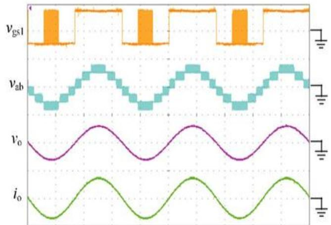
**Fig. 18. Waveforms of  $v_{gs1}$ ,  $v_{ab}$ ,  $v_o$ , and  $i_o$  at 500 W**
