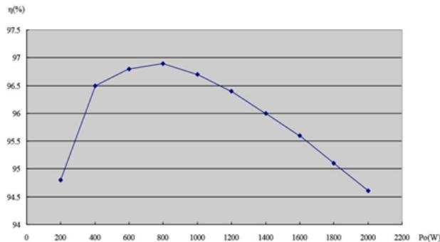
**Fig. 25. Efficiency of the proposed inverter**
