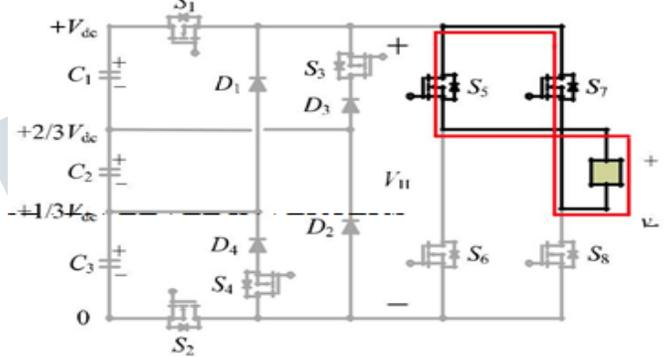
Fig. 9. Switching combination of output voltage level 0.
