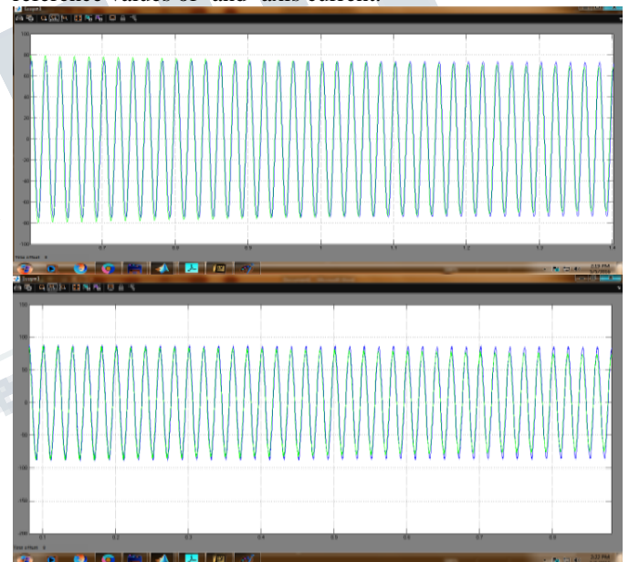
Fig. 7. Controller performance during the single-line-to-ground fault.
