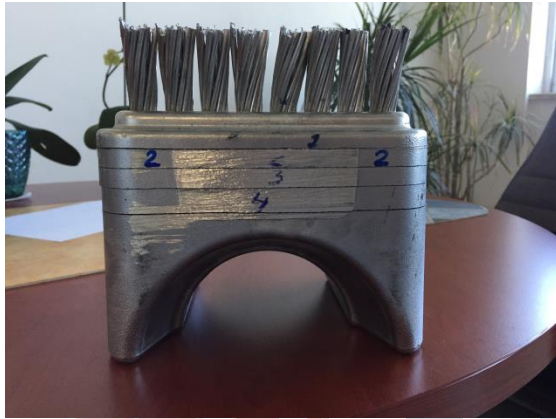
Figure 3: Sectioned sample connector (front view)
