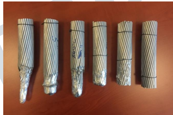
Figure 2: Temperature test for aluminum conductors
