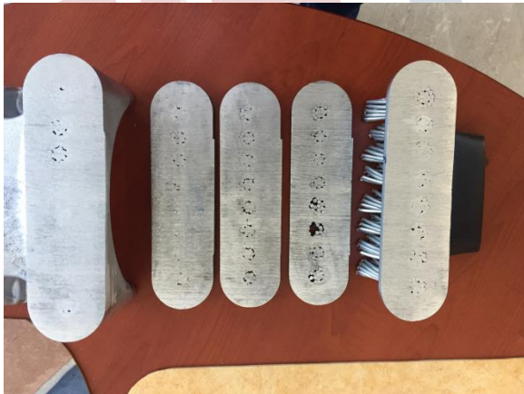
Figure 4: Sectioned sample connector (cut-away parts)
