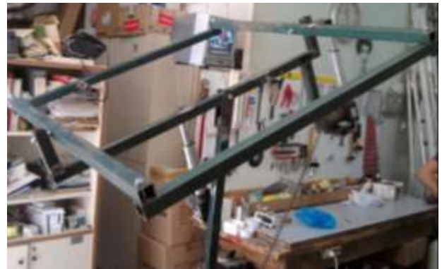
Figure 7: Dual-axis solar tracker stand with pair of linear actuators
