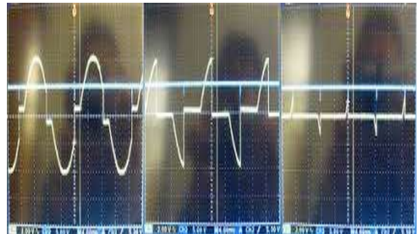
FIG: RMS Voltage Varying at different firing angle
