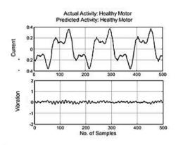
Figure : 5. Results of fault detection and isolation for healthy motor condition
