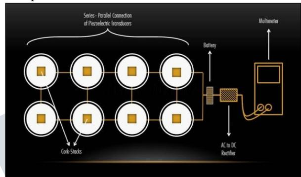
**FIG.3 SERIES PARALLEL CONNECTIONS OF PIEZOELECTRIC DISCS [7]**
