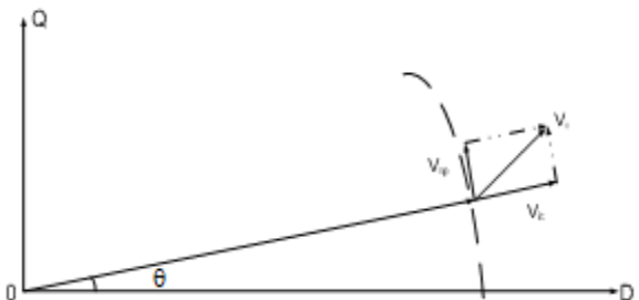
Fig. 6 Normal and Tangent part of selected voltage vector regarding stator flux vector
