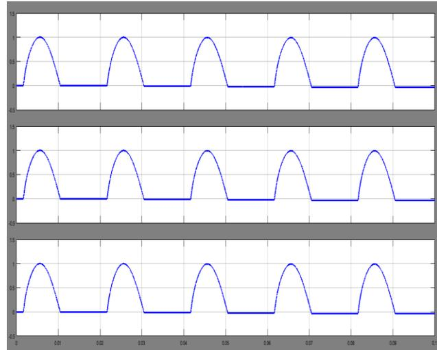
**Fig 6. Current waveform during no fault.**
