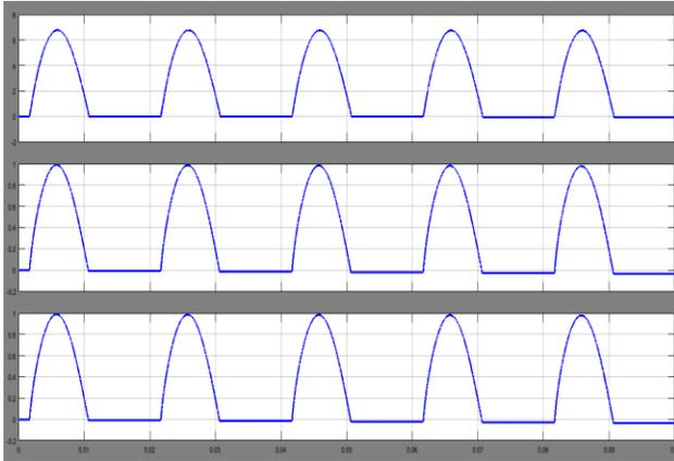
**Fig 8. Current waveform during L-G fault condition**
