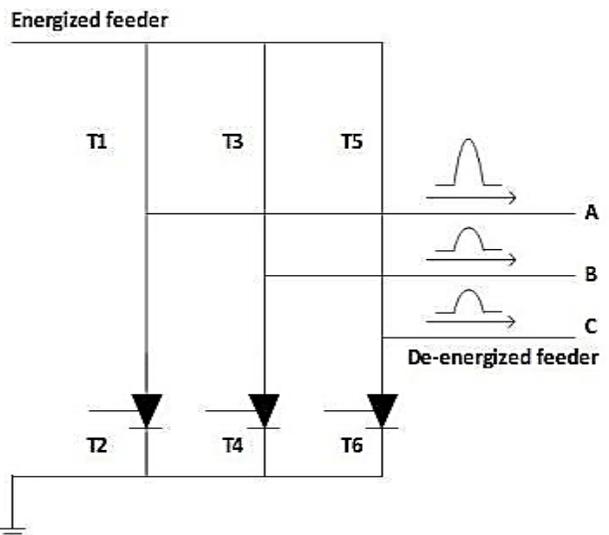
**Fig 7. Current waveform during L-G fault condition**
