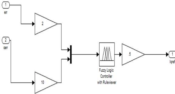
**Fig.3 Fuzzy Logic Controller (Designed)**
