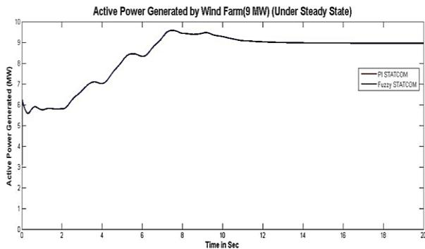
**Fig. 4 Active Power Demand under steady state condition**
