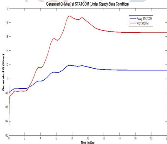
**Fig. 5 Reactive Power Demand under steady state condition**
