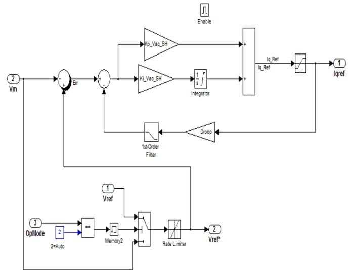
**Fig.1 PI Controller connected in STATCOM**
