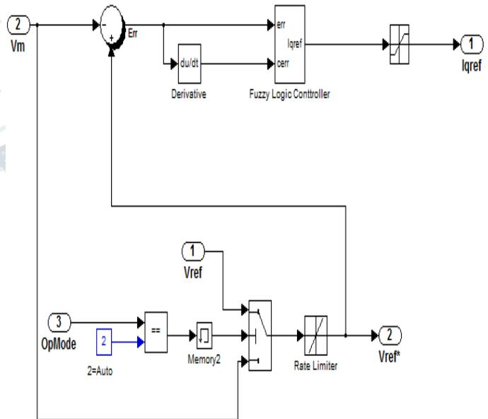
**Fig. 2 Fuzzy Logic Controller connected in STATCOM**
