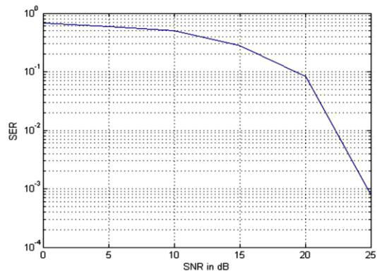
Figure 2.6 Simulated BER with 1/2-rate convolution coding
