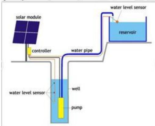
**Fig. 4:- DC submersible pump**
