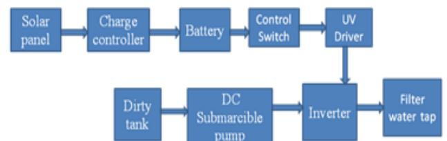
**Fig.1:- Block Diagram of Solar Water Purification**
