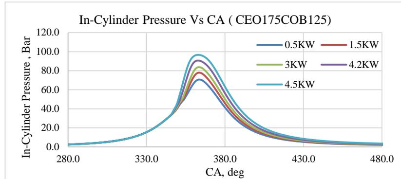
**Figure 10 In-Cylinder Pressure with CA Comparison**
