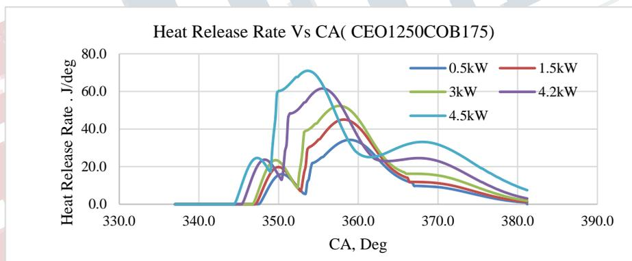
**Figure 7 Heat Release Rate with CA Comparison**
