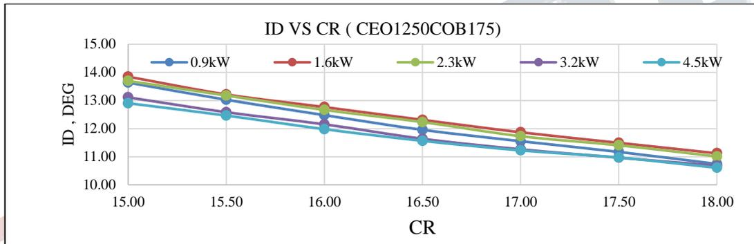
**Figure 2 ID comparison of experimental results with CR**
