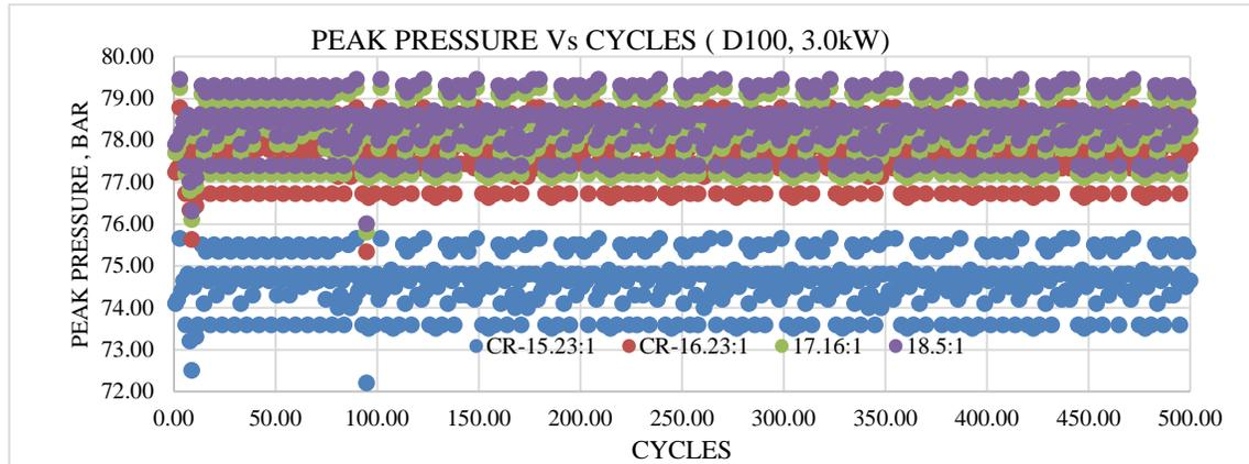
**Figure 12 Comparison of Peak Pressure of D100, and Variation for Different Compression Ratio**
