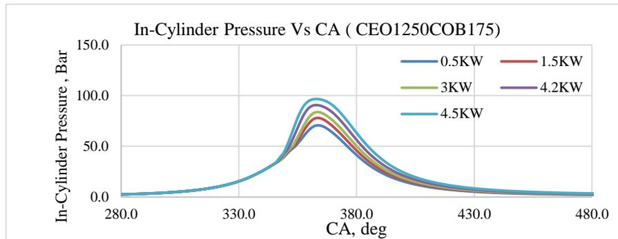
**Figure 6 In-Cylinder Pressure with CA Comparison**
