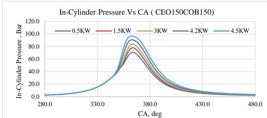
**Figure 8 In-Cylinder Pressure with CA Comparison**
