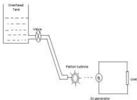
**Fig (a) micro hydro plan**
