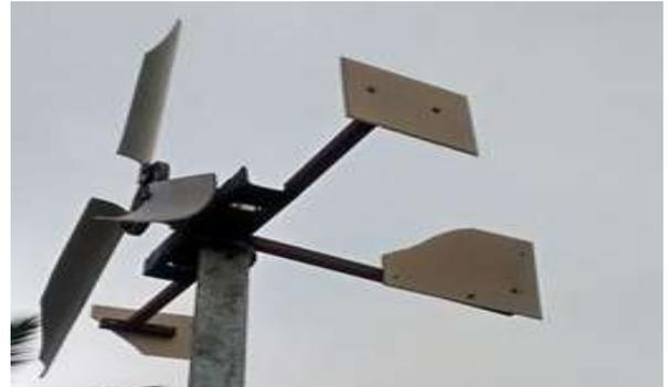
**Fig3 The three vanes for wind direction**
