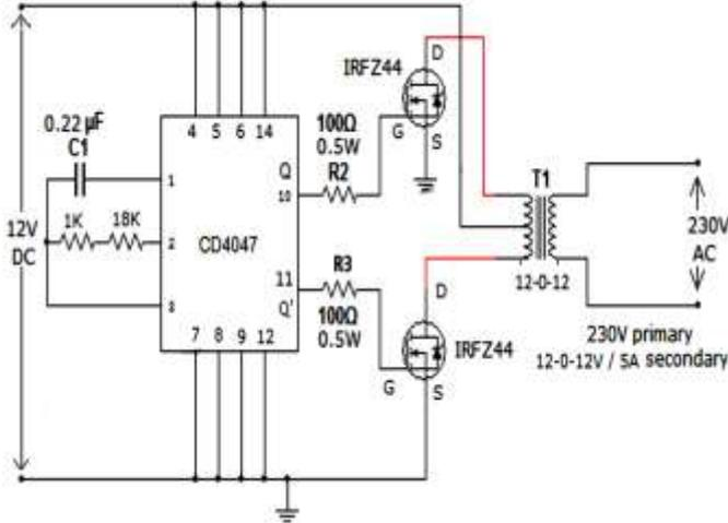
**Fig -3: Circuit diagram of DC to AC Inverter**
