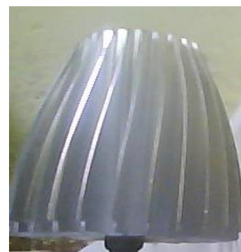
Fig 3 – Lotus type wind turbine curved aluminum blades
