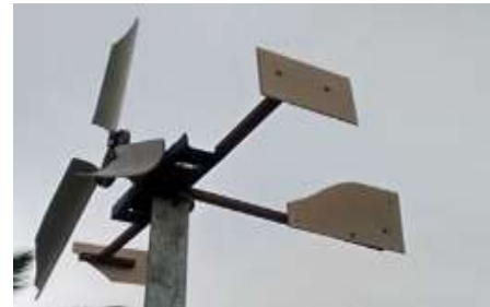
Fig3 The three vanes for wind direction
