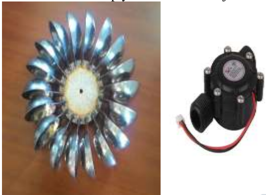
Fig -2: Pelton Turbine
