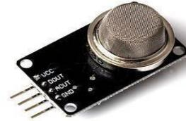
**Fig.5 Air checking purity sensor (MQ135)**
