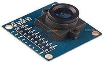
**Fig.7 Camera module (OV7670)**
