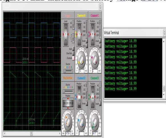
**Figure 3a: 240V square wave output near the load.**
