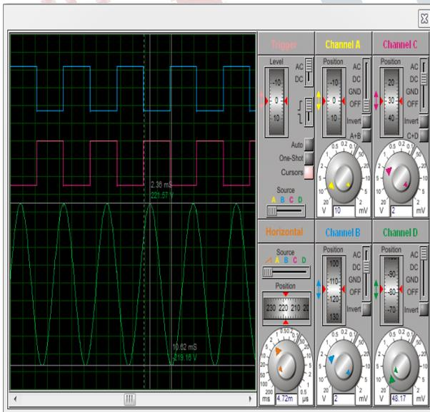
**Figure 5a: 220V pure sine wave across the load.**
