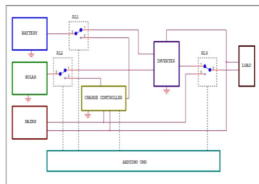
**Figure 1: Block diagram of hybrid inverter with solar battery charger.**
