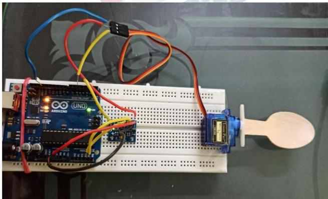
**Fig. 6 The resulting prototype of the proposed spoon**
