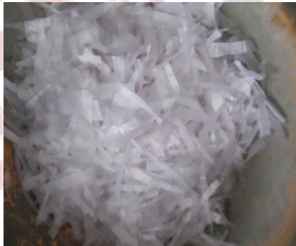
fig 1 plastic fiber used in concrete
