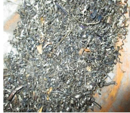
Fig 2 Lathe waste as steel fiber
