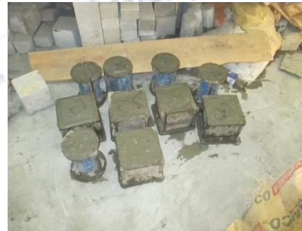
Fig 3 Concrete blocks mixed with plastic fiber and steel lathe
