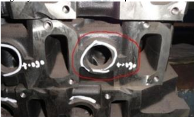
Fig.2 Oversize of bore
