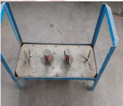
Figure 1 Special Molding systems used for Casting of Specimen.
