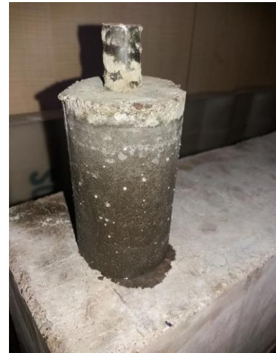
Fig 1: RC Specimen with concentrated reinforcement
