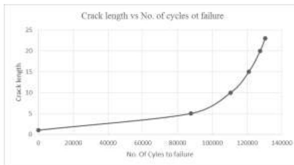
Fig. 10: Crack length vs Number of cycles to failure.
