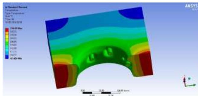
**Fig. 8: Temperature distribution of the actual die**
