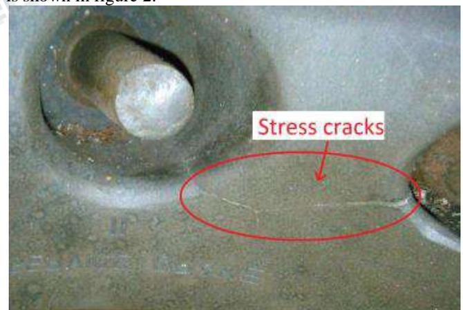
**Fig. 2: Stress cracks**
