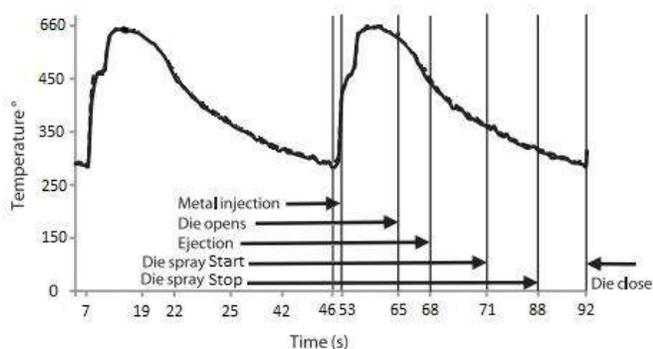
**Fig. 7: Temperature variation during the die casting process.**
