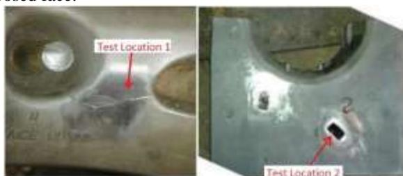
**Fig. 3: In situ metallography test location.**
