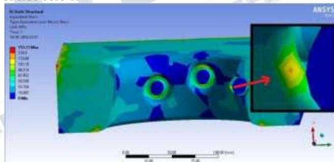
**Fig. 9: Von Mises Stress of side core 1**
