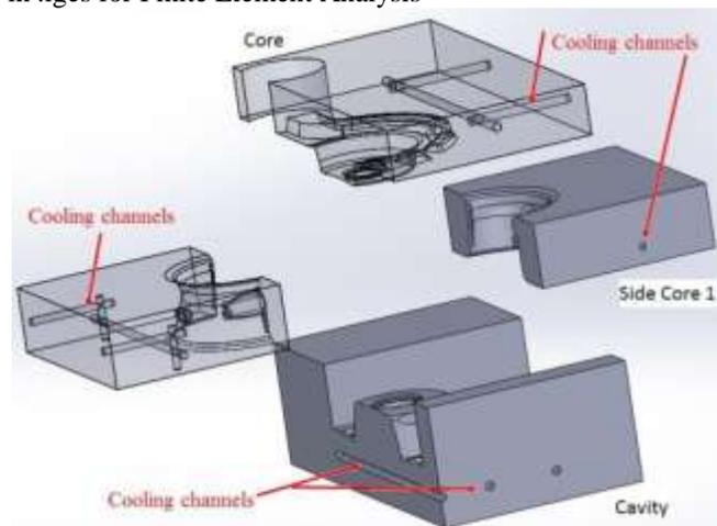
**Fig. 6: CAD model of the die**
