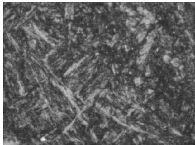
**Fig. 5: Coarse martensitic structure location 2**
