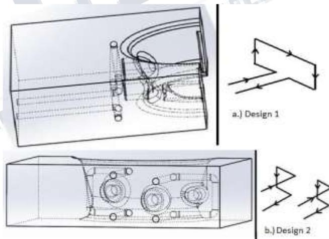
Fig. 11: New designs for side core 1
