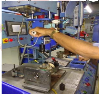
Figure 4: Poka-Yoke Voss Assembly Station Source: Pictures clicked at Knorr-Bremse CVS plant, Pune
