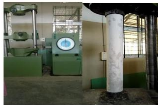
Fig: 3 Test set- up for axial loading of columns
