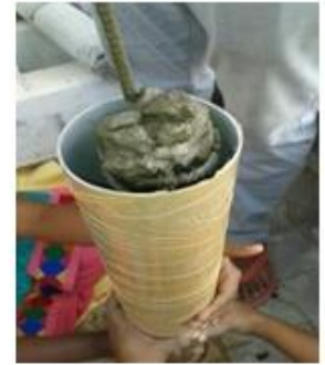
c) Placing of the concrete
