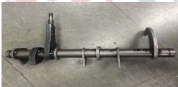
Fig. 1: Cam Shaft Mechanism Used in Circuit Breaker
