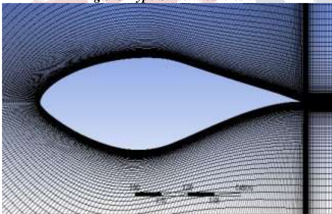
Fig.4 Grids Points Over An Airfoil
