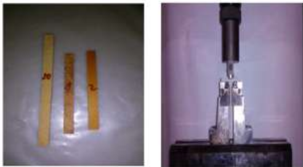
(a) Fig (a) Flexural Strength Specimen (b) Fig (b) ILSS Specimen
