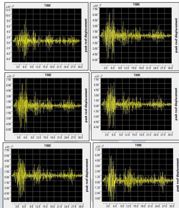
**Figure 9: Roof displacement time histories in mm v/s sec for El-Centro 1940 time history functions for a G+6 story building (a) without BRBs (b) with backward diagonal BRBs (c) with forward diagonal BRBs (d) with V BRBs (e) with cross diagonal BRBs (f) with inverted V BRBs**
