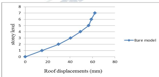
**Figure 5: Roof displacements vs. storey level for 7-storey 2D bare frame**
