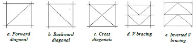
**Figure 6: Bracing configuration<sup>[16]</sup>**
