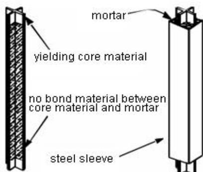
**Figure 1: Schematic diagram of buckling restrained brace<sup>[4]</sup>**
