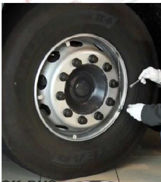
Fig: 1.1 wheel fitting section with bolts & nuts Wheel Hub Nomenclature
