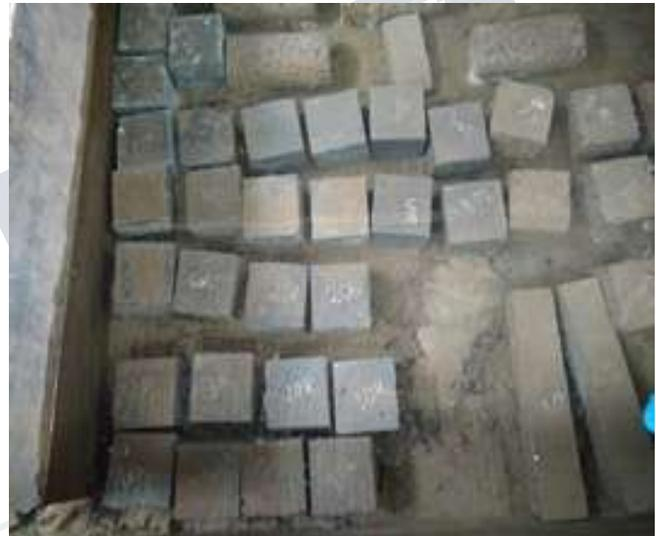
*Fig. 2. curing of samples*
