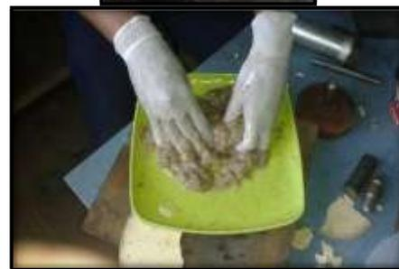
**Figure: 5.4. Resin, Hardener and Pineapple leaf fiber mixing**
