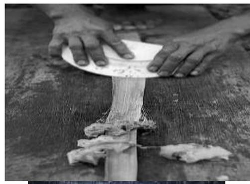
**Fig.4 Extraction of fiber using ceramic plate**
