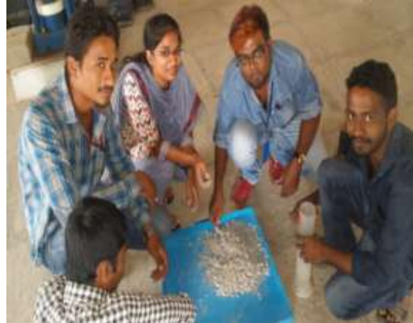
Mixing of pervious concrete with little sand
