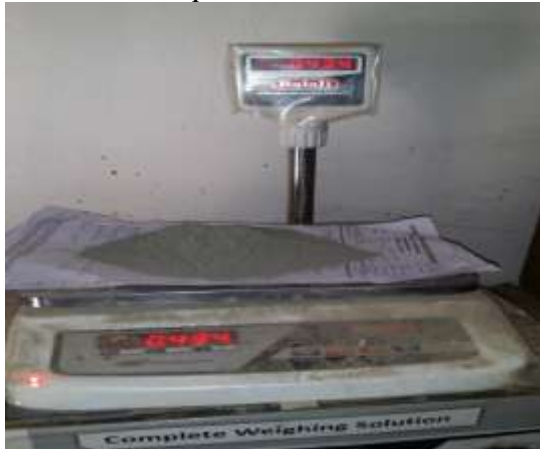
Weighing of cement(Ultra tech)
