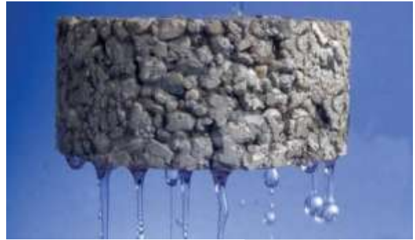
Testing of Cube that water will pass through the Cube clearly.
