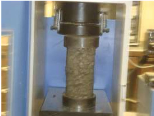
Figure 7.2: Pervious Concrete Specimen in Compression Testing Machine
