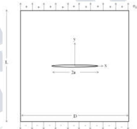
**Fig.2 Griffith Crack Model for Piezoelectric Materials**
