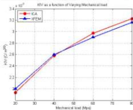
**Fig.3  $K_{IV}$  as a function of variation in mechanical load  $\sigma_{22}$  with constant electrical load of  $D_2 = 0.02$  C/m<sup>2</sup> for semi permeable crack**
