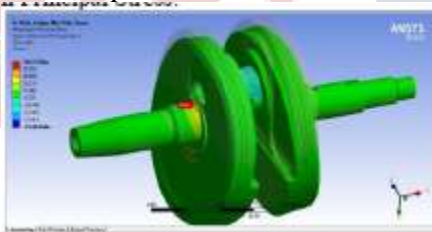
Fig 19: Contour plots of maximum principal stress induced in Crankshaft
