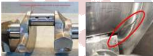
Fig 2: Failure due to bending & crack at the crankpin [9]
