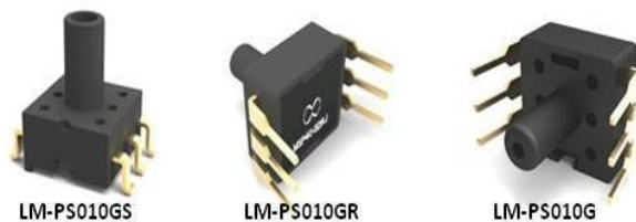
Figure3. Blood Pressure Sensor
