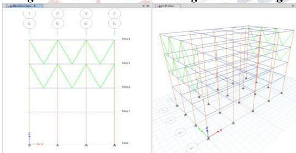
**Fig. 3 Conventional steel building with V-bracing**
