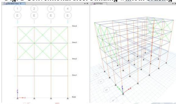
**Fig. 2 Conventional steel building with X-bracing**
