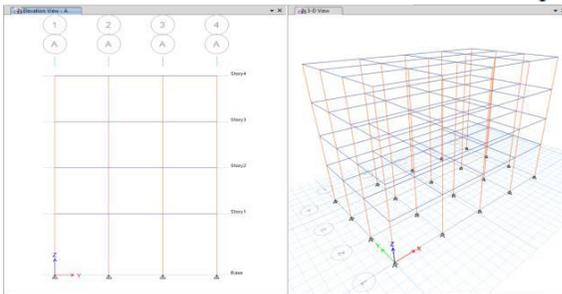
**Fig. 1 Conventional steel building without bracing**
