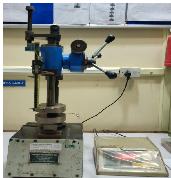
Figure 5. Helical Spring while static load test
