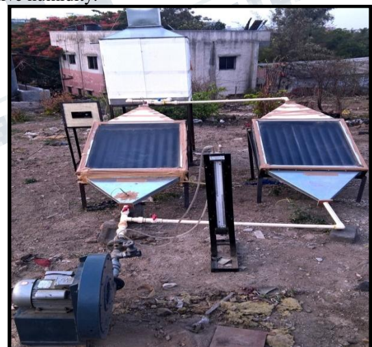
Fig. (4) Forced convection solar grape dryer with thermal energy storage [4]
