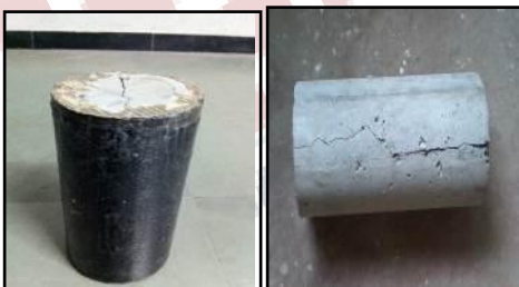
Figure 9 Failure pattern for split tensile test
