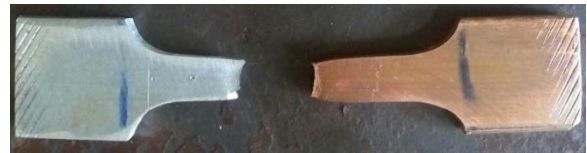
Figure: 3.6 Ultimate Tensile Specimen after Failure
