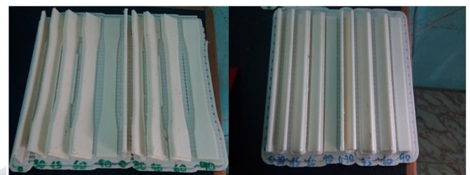
Figure 5 0,30,45,60 and 90 degree fabricated specimens in FDM machine
