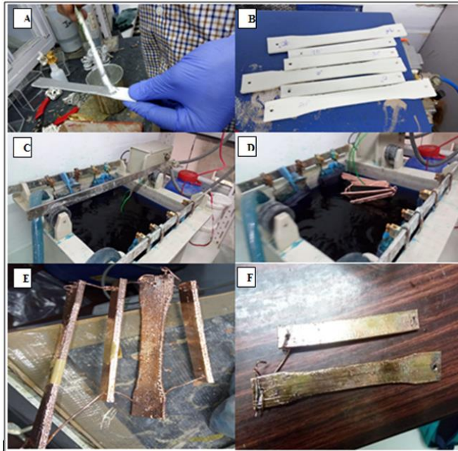
Figure 6 A. Painting conductive copper ink over plastic specimen
