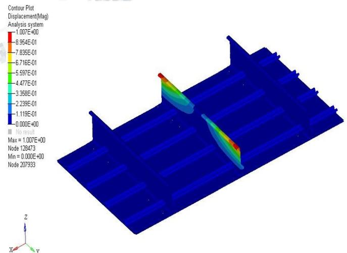
**Figure 7.1: Buckling mode plot for fuselage panel at 1g load**
