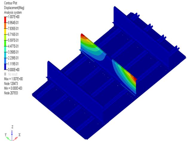
**Figure 8.2: Buckling mode plot for fuselage panel at 7g load**
