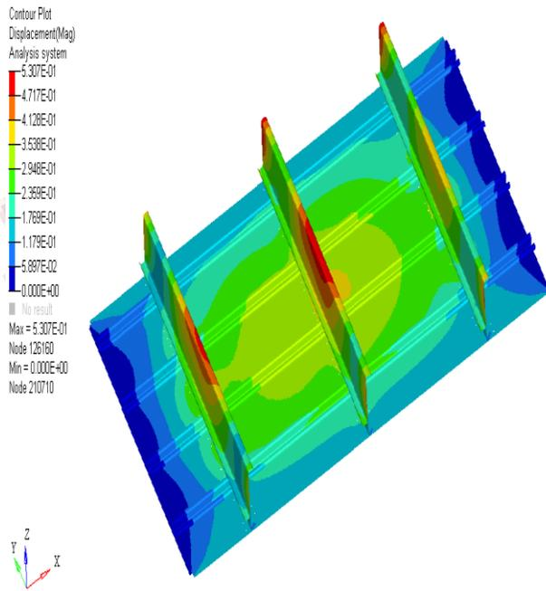
**Figure 4-1: Displacement plot for fuselage panel at 3g load**
