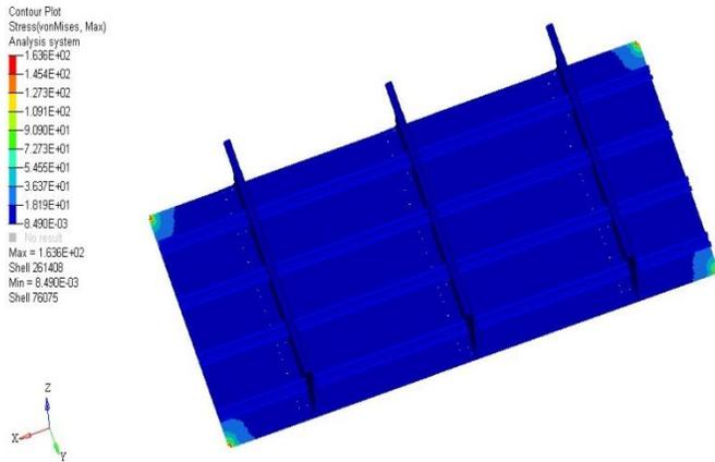
**Figure 3-2: Stress plot for fuselage panel at 1g load**
