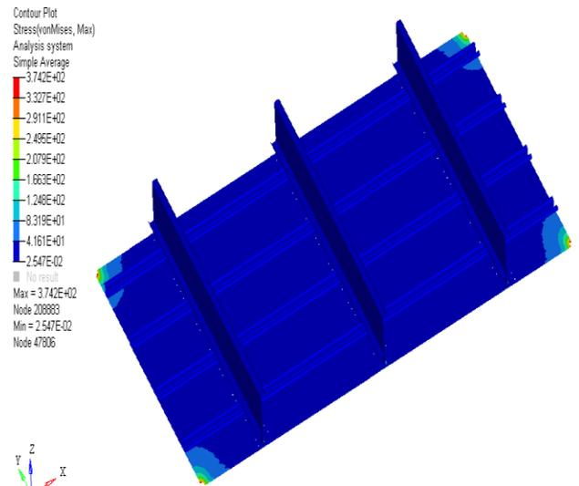
**Figure 4.2: Stress plot for fuselage panel at 3g load**
