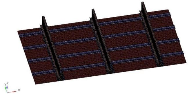
*Figure 2 - FE Model of the fuselage panel*
