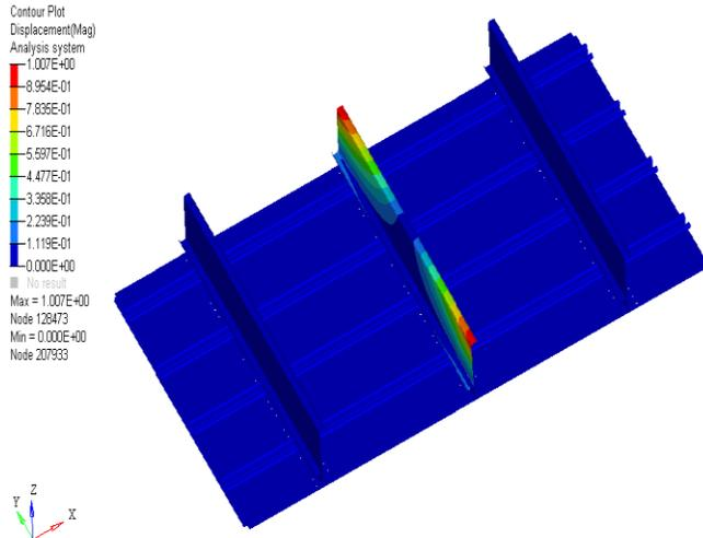
**Figure 7.2: Buckling mode plot for fuselage panel at 3g load**
