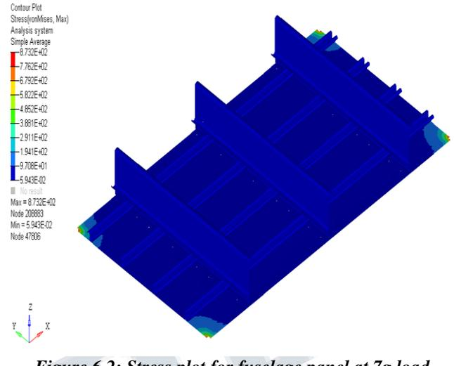
**Figure 6.2: Stress plot for fuselage panel at 7g load**
