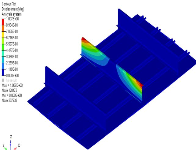
**Figure 8.1: Buckling mode plot for fuselage panel at 5g load**
