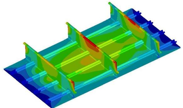
**Figure 3-1: Displacement plot for fuselage panel at 1g load**
