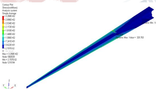
Figure 4.1: Stress Plot for I-Section for Al2024-T351
